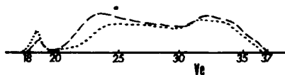
Fig. 7. Elution curves of diallyl phthalate prepolymers obtained at 250°C in N 2 atmosphere without initiator (1) and with 0.01 mol/L BPO.
